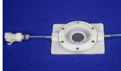
Figure 22. StageFlexer I ® for use with an inverted microscope objective
