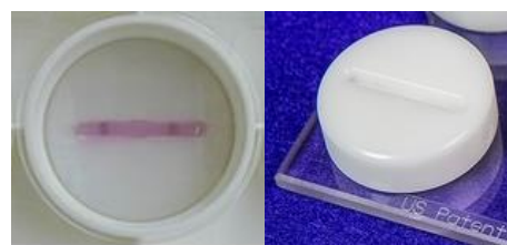
Figure 35. Representative image of 3D cell-seeded gel construct created in a Tissue Train® culture plate
