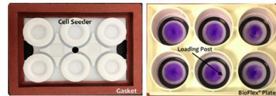
Figure 38. 6-well BioFlex® Cell Seeder station in a BioFlex® baseplate well (left picture) and the results of using a BioFlex® Cell Seeder when plating cells to confine them to the area directly above the 25 mm cylindrical loading posts, crystal violet stained cells (right picture).
