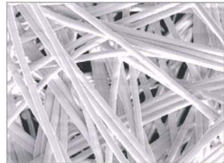
BioNOC™ II is made from 100 % PET fabrics
