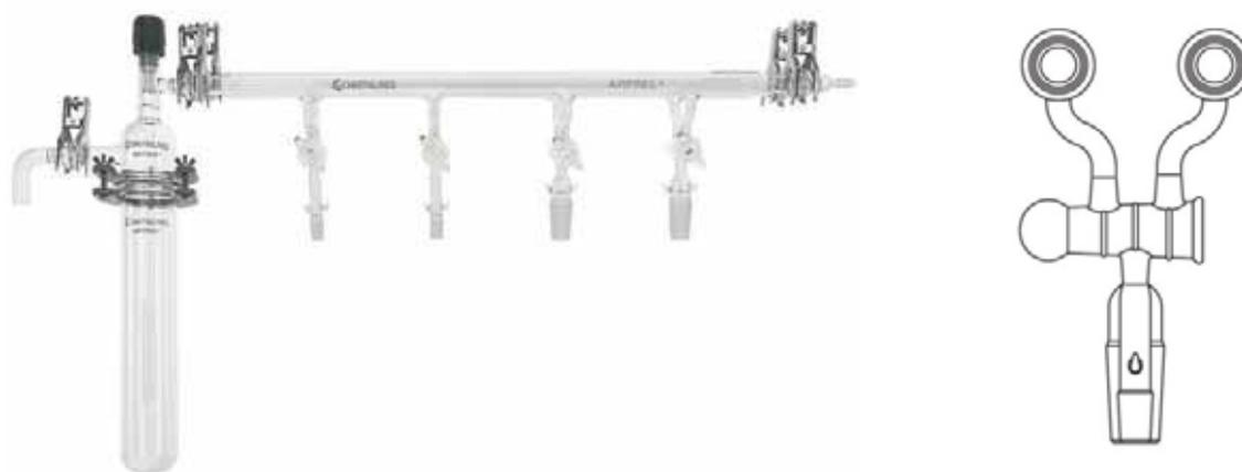
Flexible and compact, this four-ports line is constructed using 4 mm double oblique hollow high vacuum greased stopcocks on all four ports. Ports are fitted with two 14/20 inner joints and two 24/40 inner joints and are spaced 127 mm center to center.
