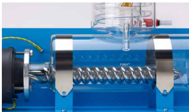
Heating element and boiler
