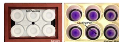
6-well BioFlex® Cell Seeder station in a BioFlex® baseplate well (left picture) and the results of using a BioFlex® Cell Seeder when plating cells to confine them to the area directly above the 25 mm cylindrical loading posts, crystal violet stained cells (right picture).
