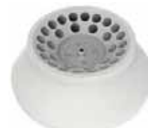
CR-43-15F-30 30 x 15 ml fixed-angle rotor, RCF 2729 g
