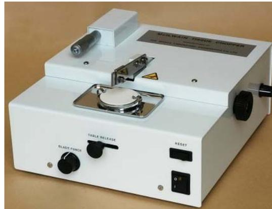
This apparatus has been designed to prepare pieces of tissue for metabolic experiments and is especially suitable for small and irregular specimens available at biopsy or from small organs. It causes much less disturbance to cell structure than homogenisers or blenders and is applicable to fragments that would be difficult or impossible to cut by ordinary methods. Typical applications are to liver, kidney and various parts of the central nervous system.
