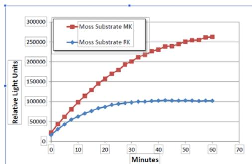
RK (Rapid Kinetic Substrate) has a strong initial activity and reaches 90 % of maximum signal after approximately 20 minutes.
