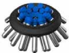
CR-43-15F-24 24 x 15 ml Festwinkelrotor, RCF 2852 g
