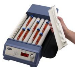
SRT6 with removable side panels and detachable roller tubes
