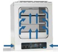
SGO: gravity convection air flow
