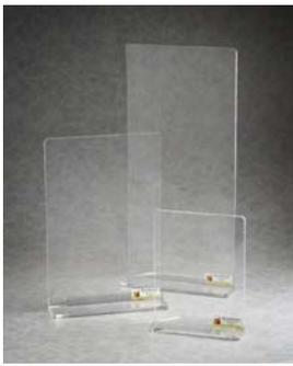
IBI Scientific Beta-Gard™ shields are manufactured using the highest quality materials to ensure safety and years of worry free service. All IBI radiation shields are constructed of 1/2" thick cast acrylic which provides the best protection against Beta radiation.
