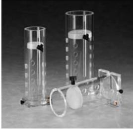
IBI Animal Restraint products are designed to hold mice and rats, keeping both user and animal safe and secure. The holders are available in five different sizes.
