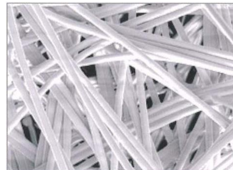
BioNOC™ II is made from 100 % PET fabrics
