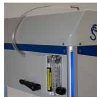
Flow control to purge the Scorpion for Chemistry
