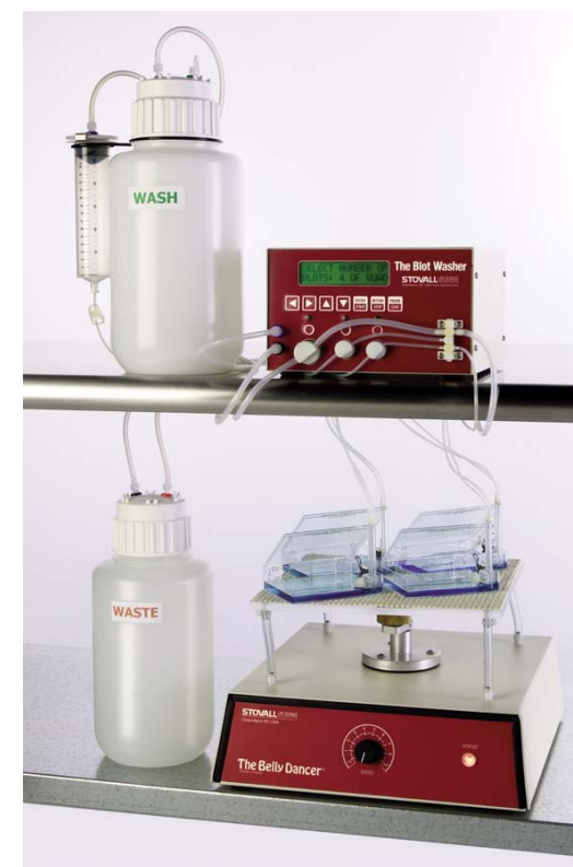
Pictured here with The Stovall Blot Washer (the automated liquid delivery and aspiration system), the Belly Dancer is the shaker of choice for washing & incubation of Western blots.
